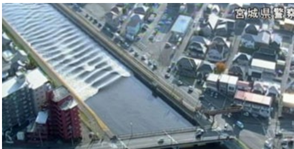
Figure 7: Standing tsunami bore wave in Sunaoshi River, Miyagi Prefecture, Japan 2016. (Miyagi Prefectural Police / Kyodo / Reuters, 2016).
