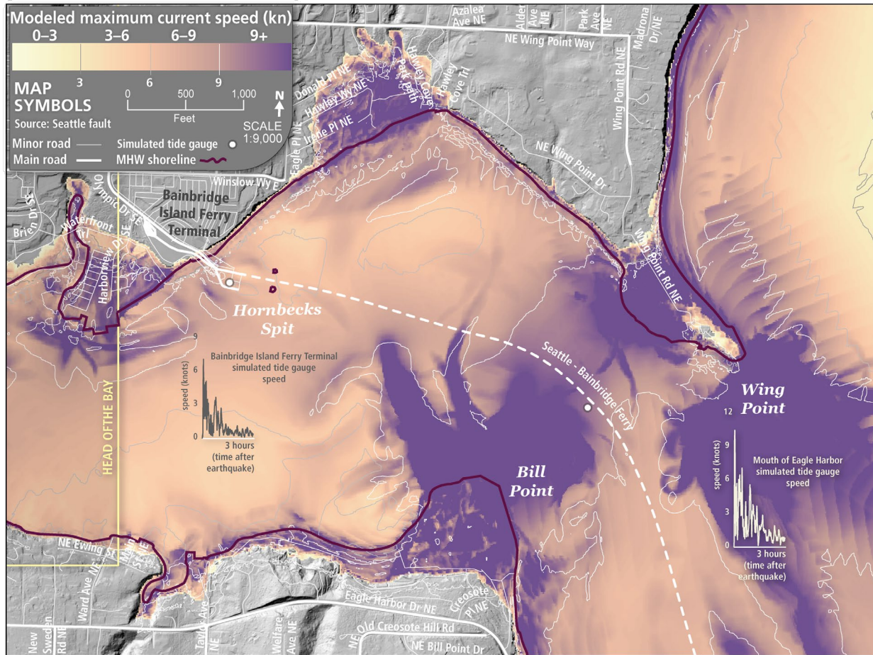
Figure 25: Modeled tsunami current speeds within the Mouth of the Bay boundary area from the Seattle Fault Zone (SFZ) earthquake scenario. Tidal datum: maximum values generated between the Mean High Water and Mean Low Water runs. Model resolution: 1/9th arc-second (3 m).
